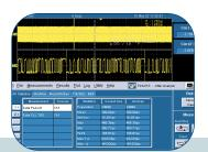
TDSJIT3 jitter analysis package rapidly characterizes the random and deterministic components of jitter in high-speed designs.
