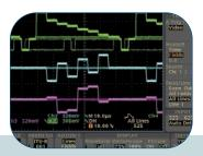
The TDS3SDI 601 serial/digital video module makes the TDS3000B Series oscilloscope a fast, tell-all tool for video troubleshooting.
